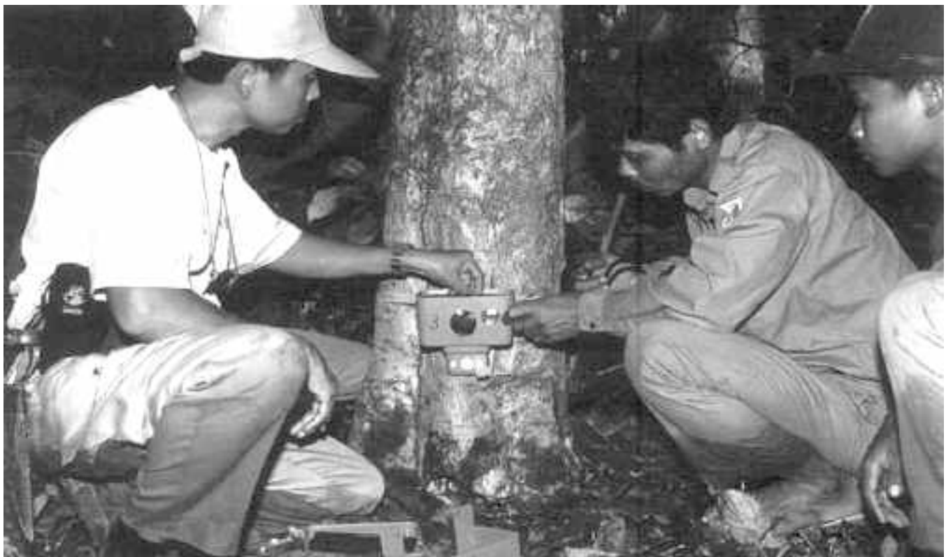
Fig. 11. Infrared - based camera - traps were used to detect the tigers and prey species.
